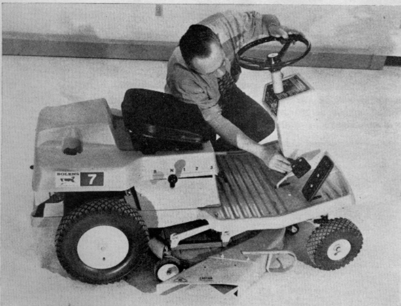
Brake pedal on seven-horse Bolens rider must be down and locked to start (left). This prevents forward motion, and declutches and brakes mower blades. Photo above shows a clever little catchpan that prevents gas from running down onto the muffler. Runover splashes on the ground.
