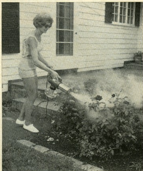
Garden fogger runs off the tractor's 36-volt pack, too. The low-voltage power system is well below the shock-hazard level.
