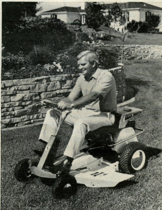
THE 5-HP SCAMP is made by Allis-Chalmers and it sells for $419. It features electric starting, a foot-controlled clutch and a 26-inch rotary mower
