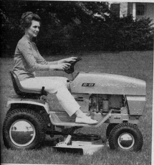
SPERRY NEW HOLLAND has upped lawn tractor line to four units. The S8 is a compact 8-hp machine that offers optional hydrostatic transmission
