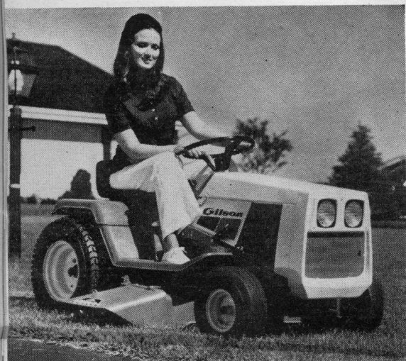
GILSON 8-HP TRACTOR has low profile and 36-inch, twin-bladed mower. Traction-drive system is said to deliver smooth power in all speeds
