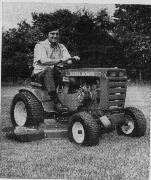
WHEEL HORSE couples a 48-inch mower to 16-hp engine in its big Automatic garden tractor (right). Attachments include hefty sweepers, snowblowers
