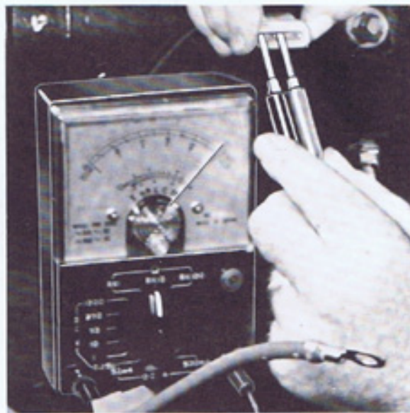
21. Multitester set on RX10 wires disconnected from motor. Approximately 16 ohms reading on multitester from wire 62 to wire 22 on plug 3 connecting the motor field is normal.
