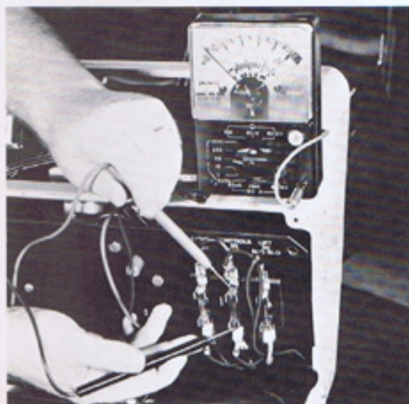
7. Multitester reads 0-volts across fuse holder when fuse is good and in the holder.
