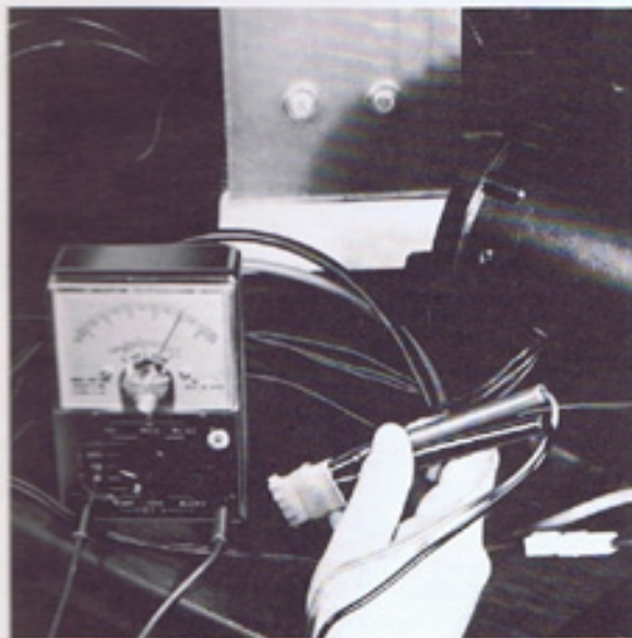
19. Multitester reads 36-volts in first three speeds on wires 62 and 22 on Plug 3 connecting the motor field.
