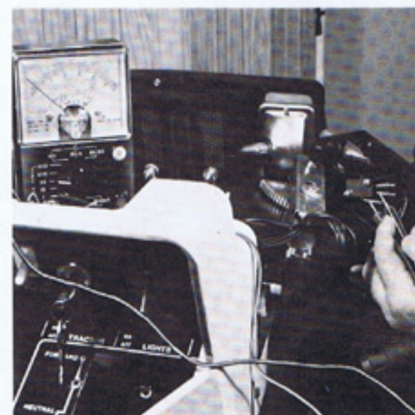
12. Multitester reads 0-volts across wires 16 and 41 to the reverse switch terminals when speed control is in the reverse position (switch is closed).
