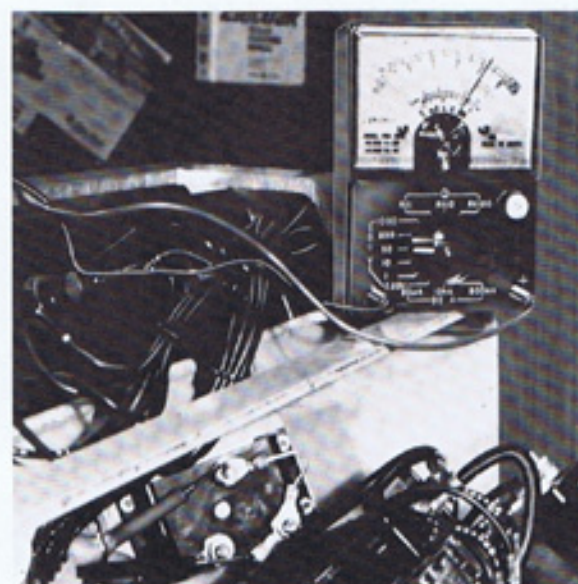
10. Multitester reads 36-volts across power disconnect terminals when power disconnect is out.
