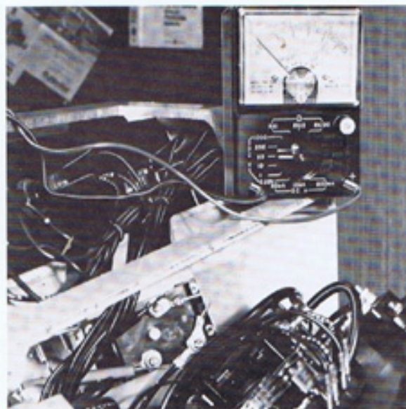
9. Multitester reads 0-volts across power disconnect terminals when power disconnect is engaged.
