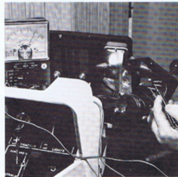
11. Multitester reads 36-volts across wires 16 and 41 to the reverse switch terminals when speed control is in a forward position (switch is open).
