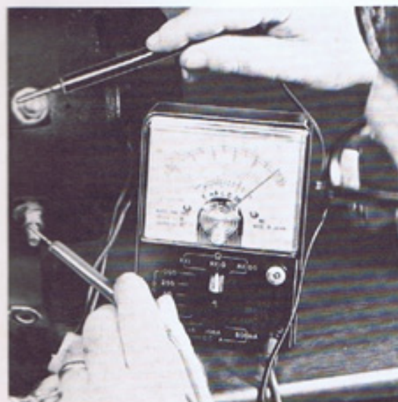
20. Multitester set on RX10 wires disconnected from motor. Full-scale deflection on multitester across motor armature terminal is normal.
