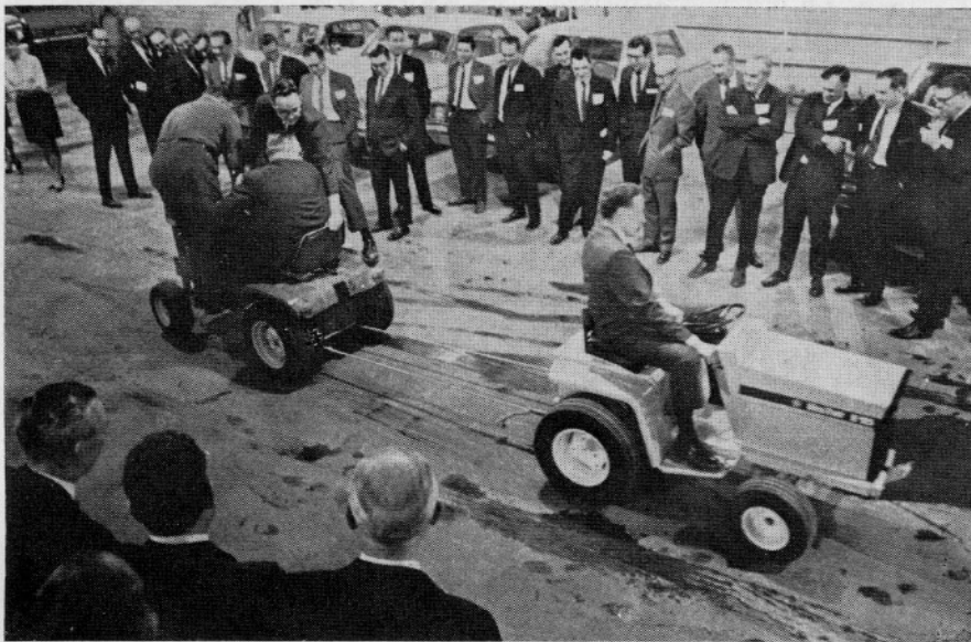
Tug-of-war is easily won by Elec-Trak. Additional weight of two extra men for better traction did not help gasoline-engine powered tractor of comparable size on left
